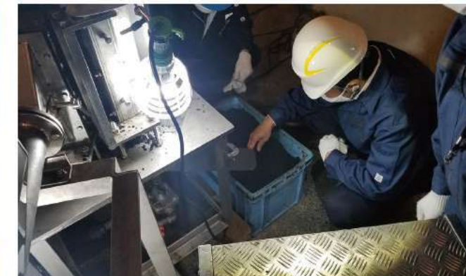
Full-scale demonstration testing of the conversion of sludge generated in the purification treatment process into fuel started from October in 2020. The sludge left over from the dehydration of organic liquid waste will be desalinated and dried and turned into solid fuel to replace fossil fuels. The company aims to start production with annual capacity of 5,400 tons in FY2023.
